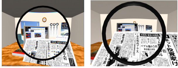
Figure 12. Examples of per-vertex refraction using a convex lens model (left) and a concave lens model (right).
