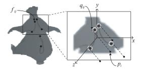
Figure 2. The diagram of the estimating function. The value of the estimating function is decided by using the distance between the 2D feature point  $f_{ij}$  and the projected 2D point  $q_{ij}$ of its corresponding 3D feature point  $p_i$  by applying  $R_j$  and  $s_j$ . ©Disney
